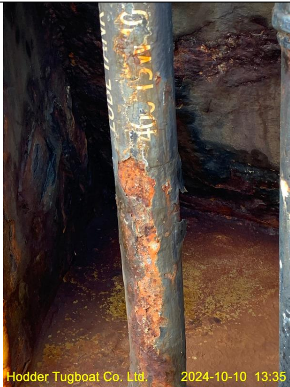
Rusted lube tank pipes and vent/air pipes
