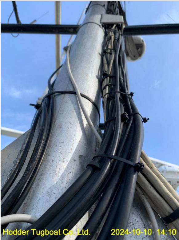
Organized wiring of the mast
