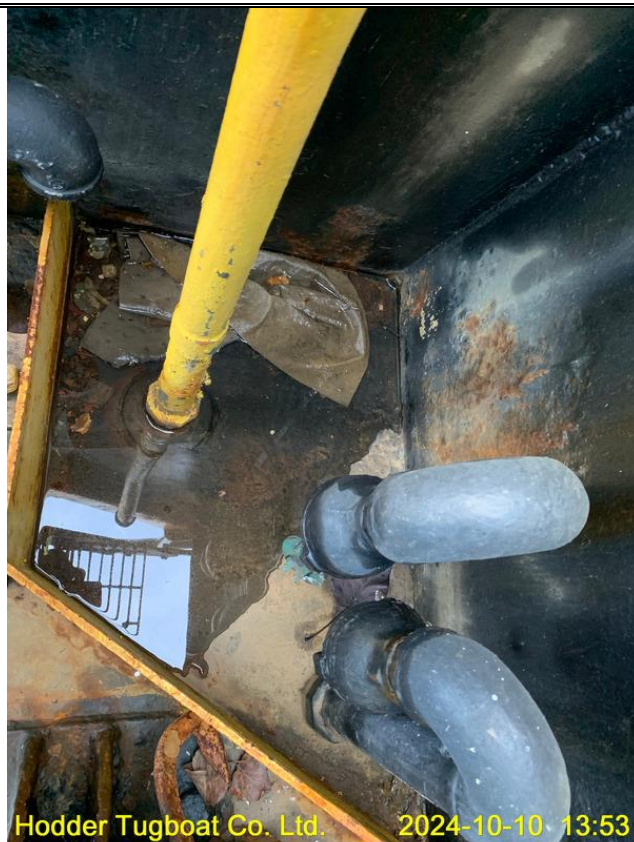
Bunkering piping section and oil spill area
