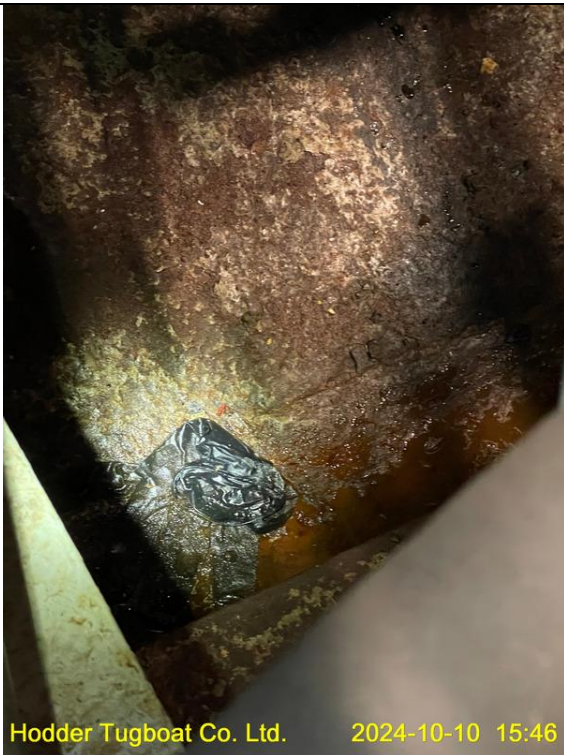
Rusty section of a hull
