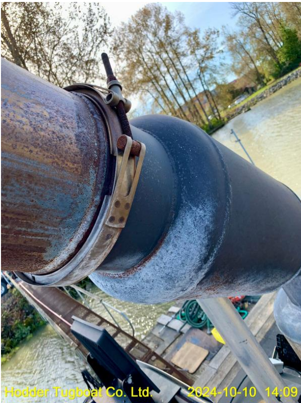
Close-up rust on an exhaust pipe
