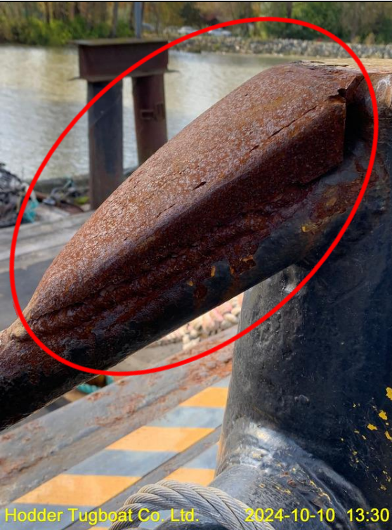
The boat's substantially rusted bollard mount
