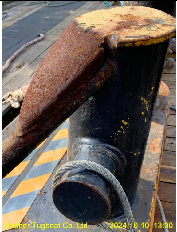
The boat's substantially rusted bollard mount
