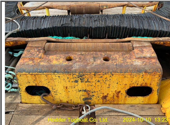
Rusted fairlead roller and foundation
