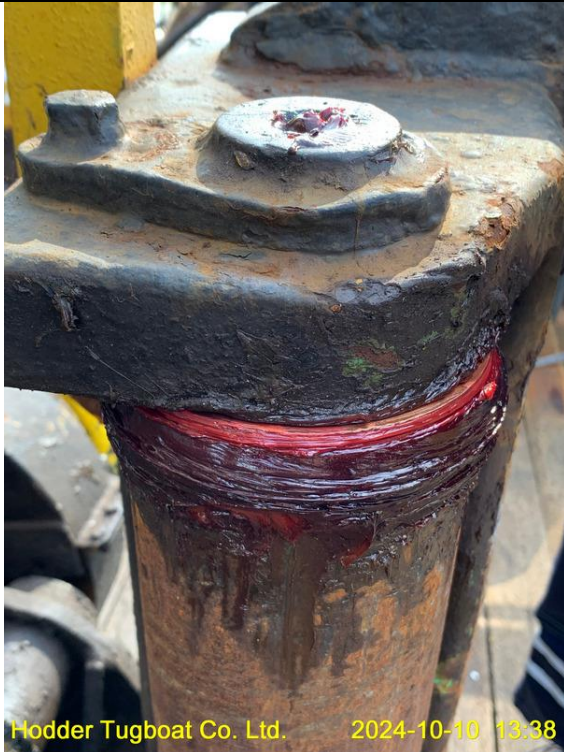
Properly greased lead roller of the towing winch
