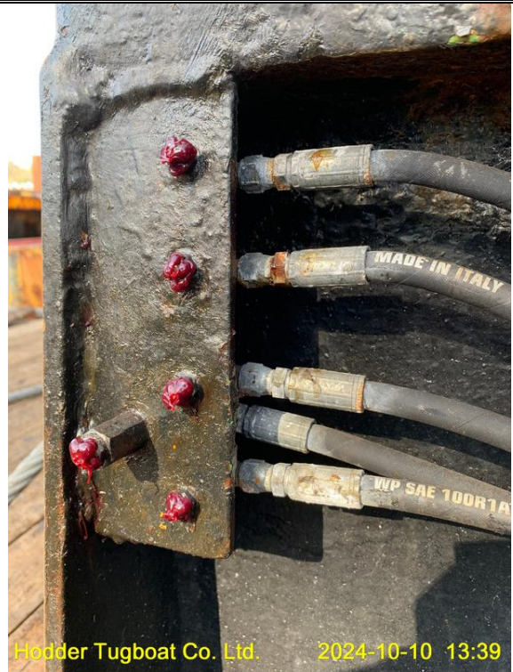
Hydraulic fluid pipes for the braking system
