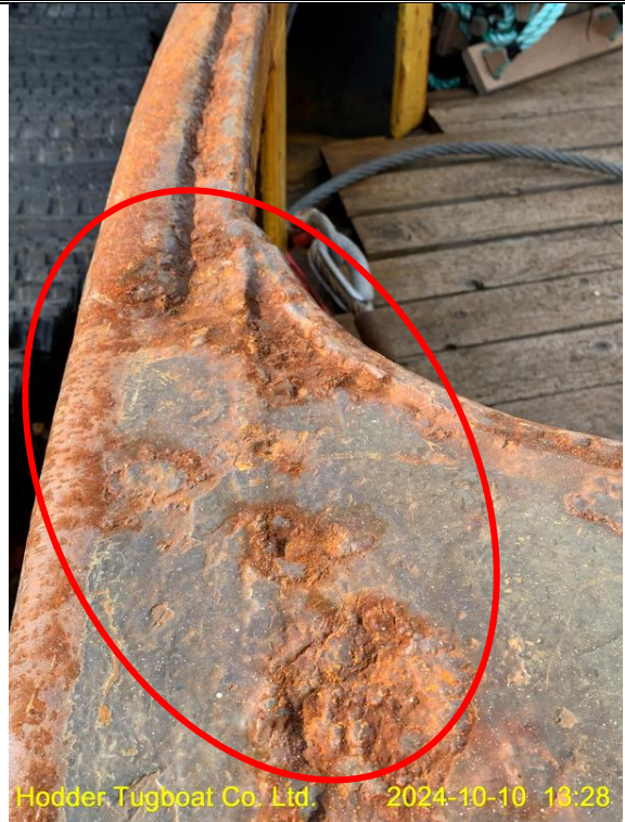
The rusted and visibly pitted starboard side of the boat
