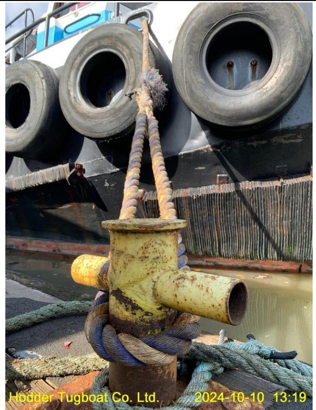
Berthed tugboat with nylon rope to mooring bollard
