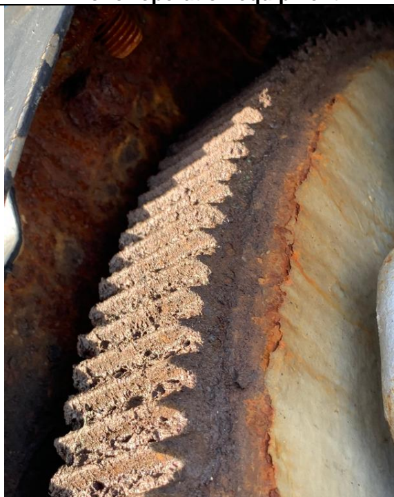
Corrosion on the cogwheel
