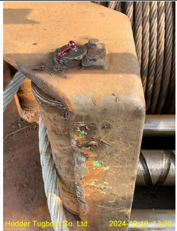
Properly greased lead roller of the towing winch
