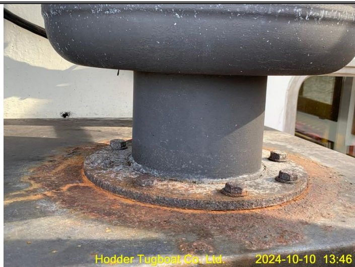
Rusty exhaust pipe mounting
