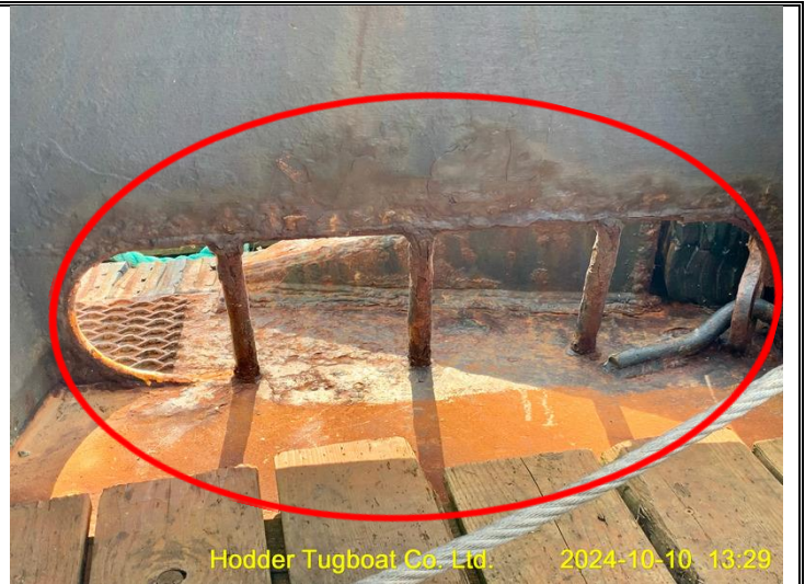
Rusted waterway of the boat's deck
