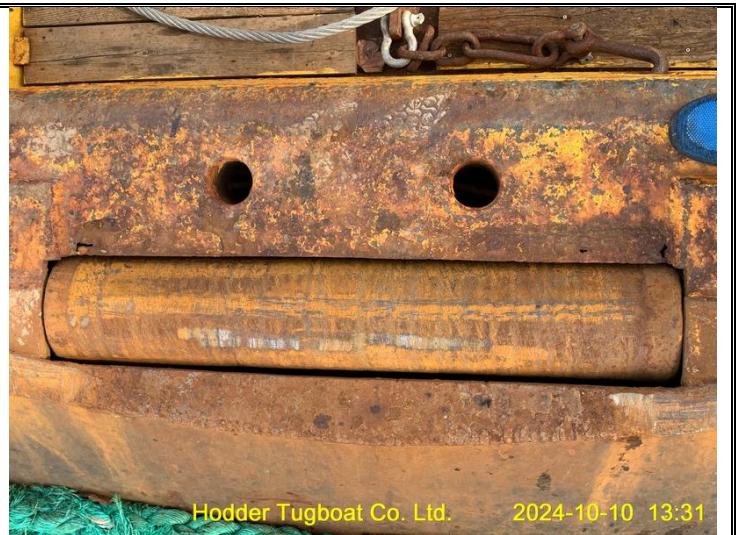
Rusted fairlead roller and foundation
