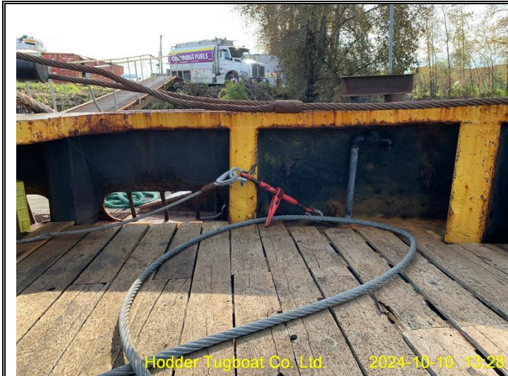
Rusted waterway of the boat's deck
